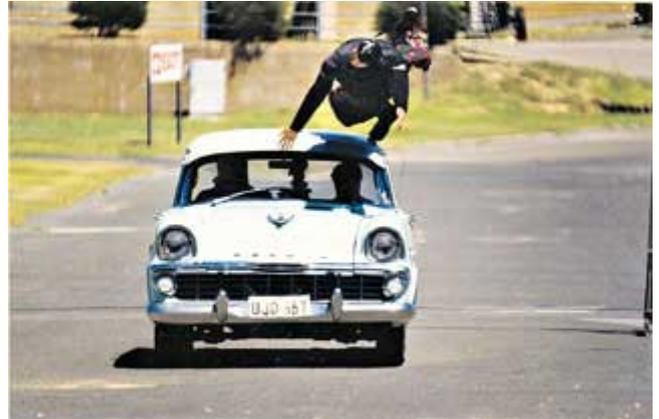
*A pedestrian crash test using a biomedical dummy. The dummy impacted the leading edge of the car; the head dented the bonnet, there was impact with the sunvisor and roof, and the dummy landed heavily on the road, then bounced along the road. In this test at 56kmh the body was projected "down range" 27 metres.*
